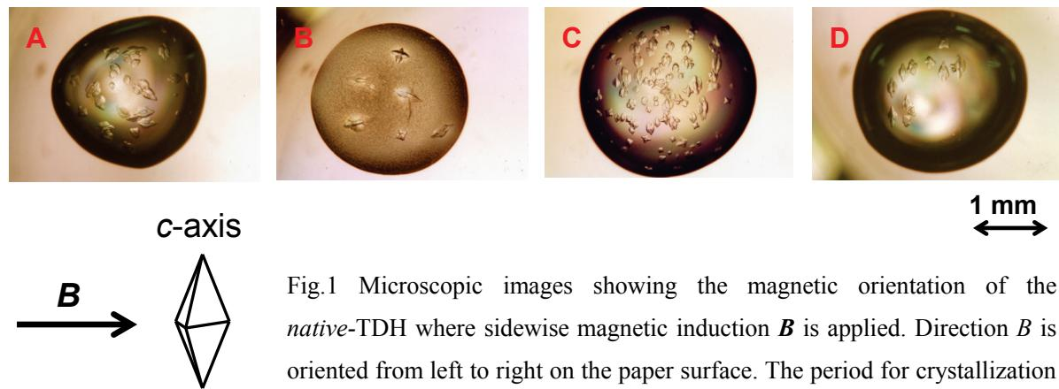
Fig.1 Microscopic images showing the magnetic orientation of the *native*-TDH where sidewise magnetic induction *B* is applied. Direction *B* is oriented from left to right on the paper surface. The period for crystallization is 3 days, and the temperature is 5°C.
